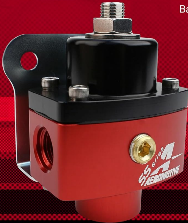
Figure 2: Overview of the SS-Series ORB-06 Carburetor Fuel Pressure Regulator, detailing its suitability for carbureted street or racing engines on gasoline, adjustable base pressure (5-10 PSI), and dead-head design for up to 750 FWHP.
