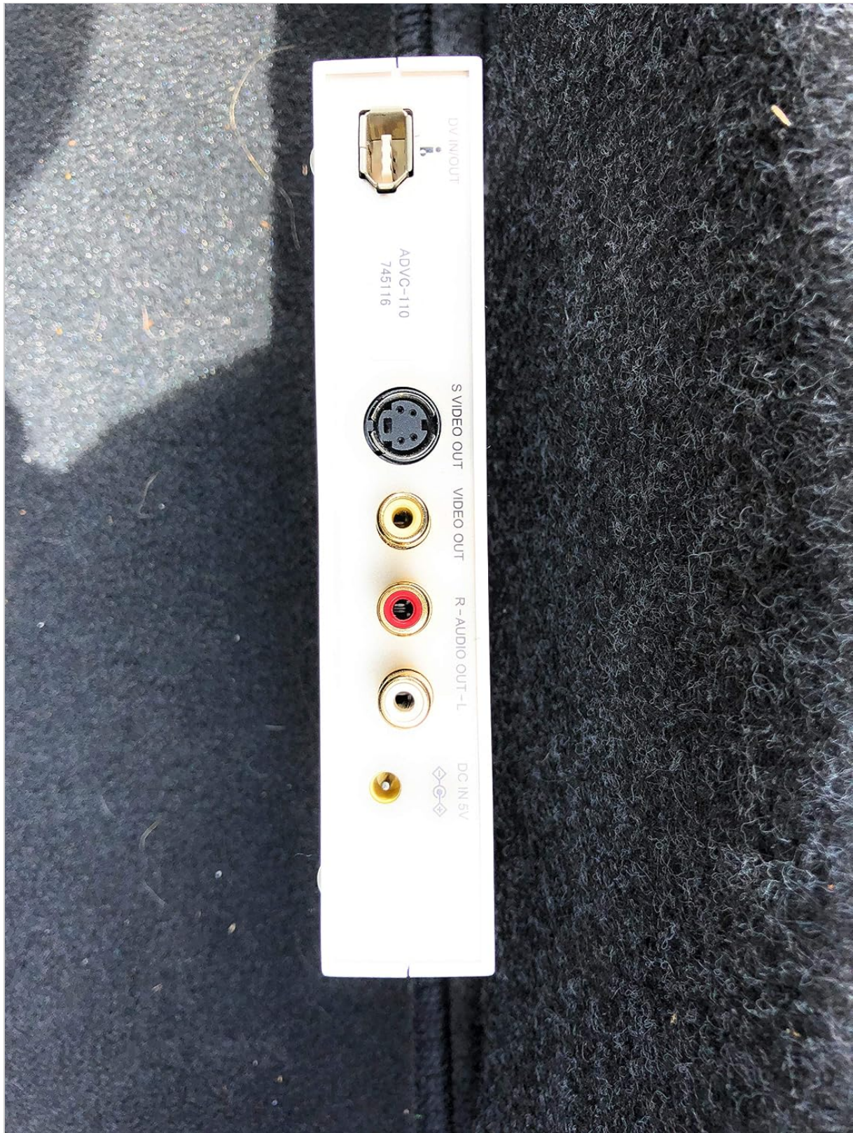
Figure 1: Rear view of the ADVC-110 showing the DV IN/OUT, S VIDEO OUT, VIDEO OUT, R-AUDIO OUT-L, and DC IN 5V ports.
