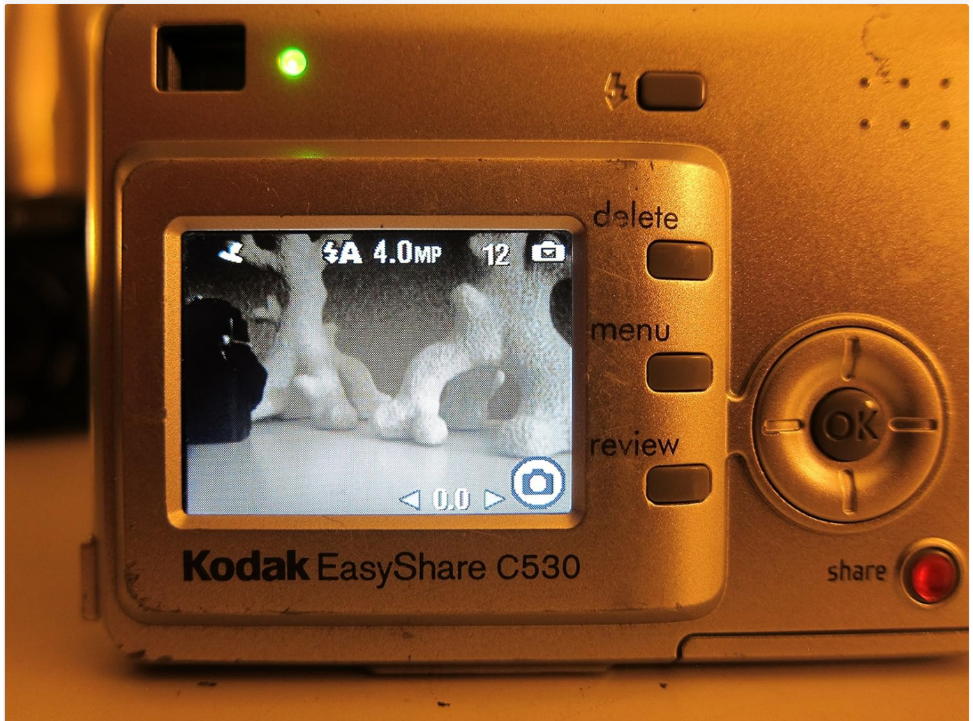
Rear view of the camera, showing the LCD screen and navigation buttons for reviewing media.
