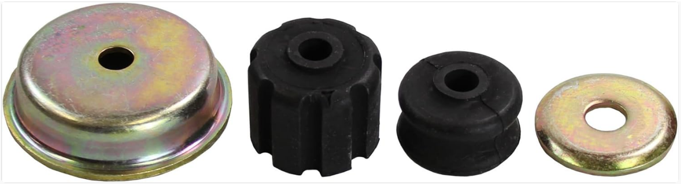
Figure 3.1: Individual components of the Monroe Strut-Mate 902978 Suspension Strut Mount kit. This includes a washer, a cup, an upper bushing, and a lower bushing, designed for direct replacement.
