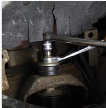
Figure 4.2: Detail of a wrench being used to tighten a suspension nut during installation.
