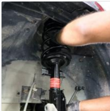
Figure 4.3: A strut assembly being carefully positioned for installation into the vehicle's wheel well.
