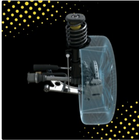
Figure 5.1: An animated diagram illustrating the dynamic movement of a vehicle's suspension system, where the strut mount plays a key role in stability and comfort.
