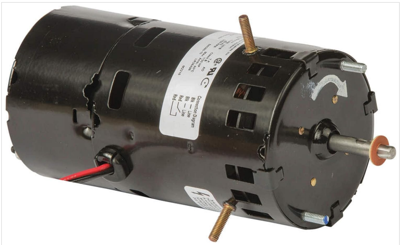
Figure 1: Fasco D454 Blower Motor. This image shows the black cylindrical motor with ventilation slots. The shaft with a washer and mounting studs are visible. A label on the motor displays the connection diagram: two Black wires for Line, and two Red wires for the other connection. An arrow indicates clockwise rotation.
