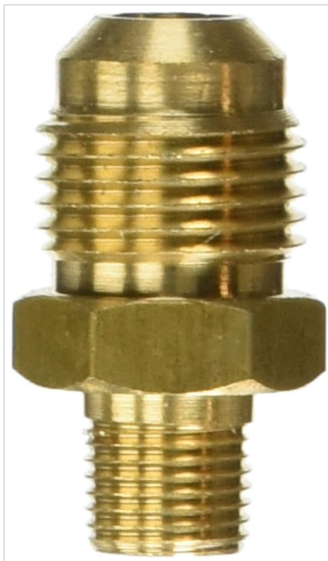
Image 1.1: The Bayou Classic 5235 Orifice Connector, a brass fitting with threaded ends and a hexagonal section for wrenching. It features a 3/8-inch flare male connection on one end and a 1/8-inch male NPT connection on the other, with an internal #57 orifice.
