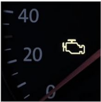
Figure 6: A close-up of a vehicle dashboard showing the illuminated Check Engine Light. This light indicates a potential issue with the engine or emissions system that requires attention.
