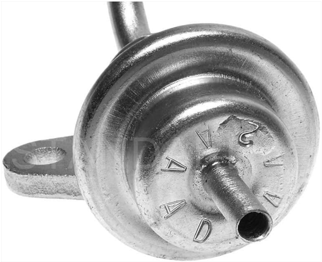
Figure 3.2: Top view of the PR280 Fuel Pressure Regulator. This perspective highlights the vacuum port, which connects to the engine's intake manifold to sense pressure changes.
