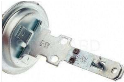
Figure 2: Another view of the VC250, highlighting the integrated mounting bracket and the arm that connects to the distributor's breaker plate.
