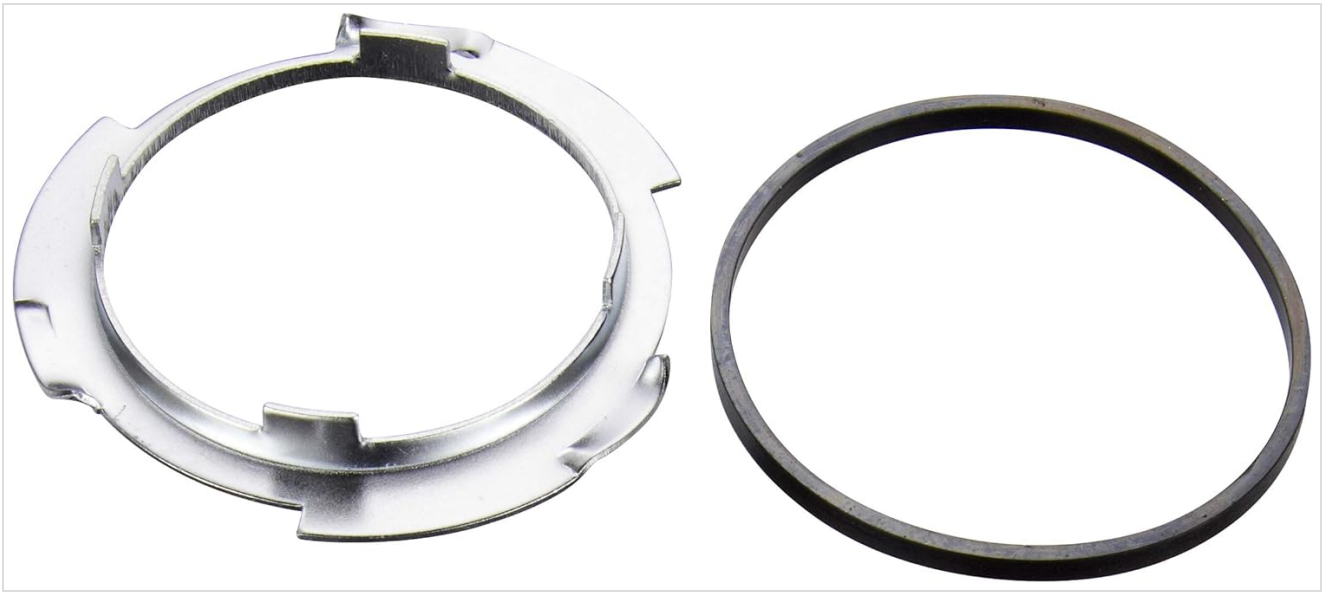
Image: The new gasket and locking ring, essential components for sealing the fuel sending unit to the tank. Secure the unit with the new locking ring, ensuring it is tightened evenly to create a proper seal. Do not overtighten.
