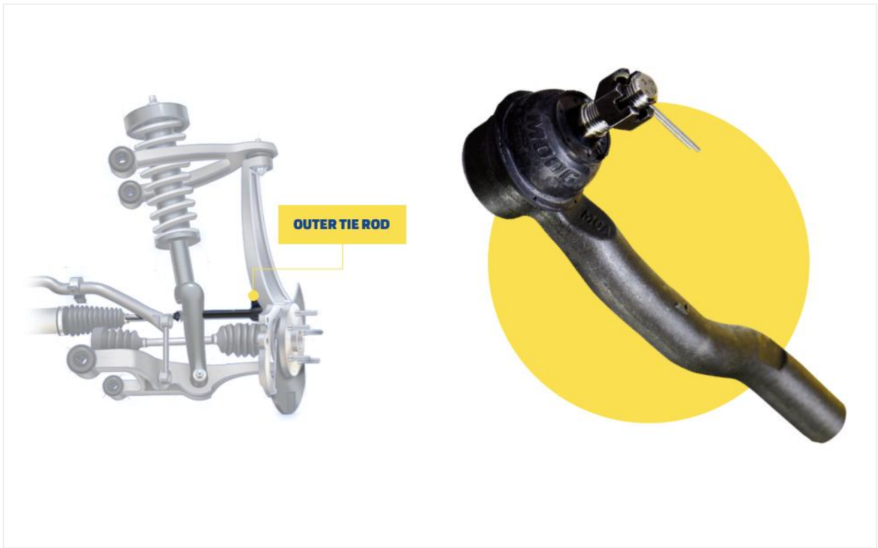
Figure 6.2: Outer Tie Rod Location, illustrating its position within the steering assembly.
