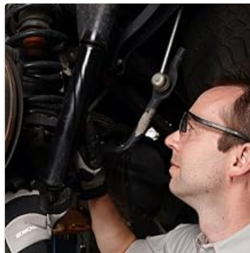
Image: A technician inspecting suspension components during the installation process.
