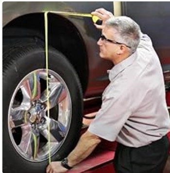
Image: Measuring vehicle ride height, a key maintenance check for air shocks.
