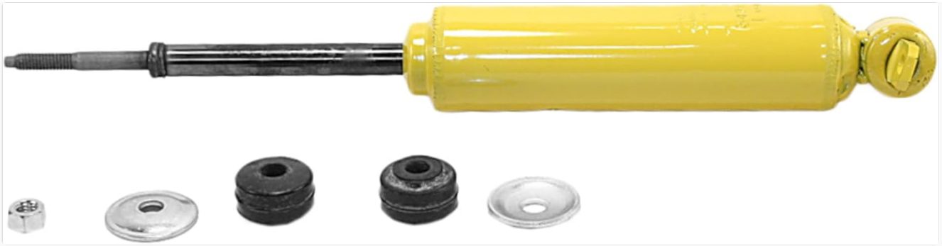
Figure 1: Monroe Gas-Magnum 34741 Suspension Shock Absorber and included hardware.
