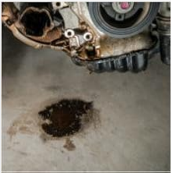
Image: A visual representation of an oil leak on the ground, indicating a potential issue with the oil pan gasket or surrounding components.
