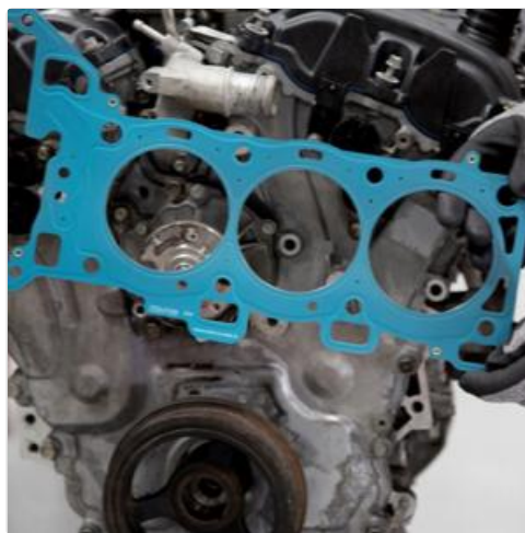
Image: A person wearing gloves holds a blue head gasket over an engine block, illustrating the placement process.
