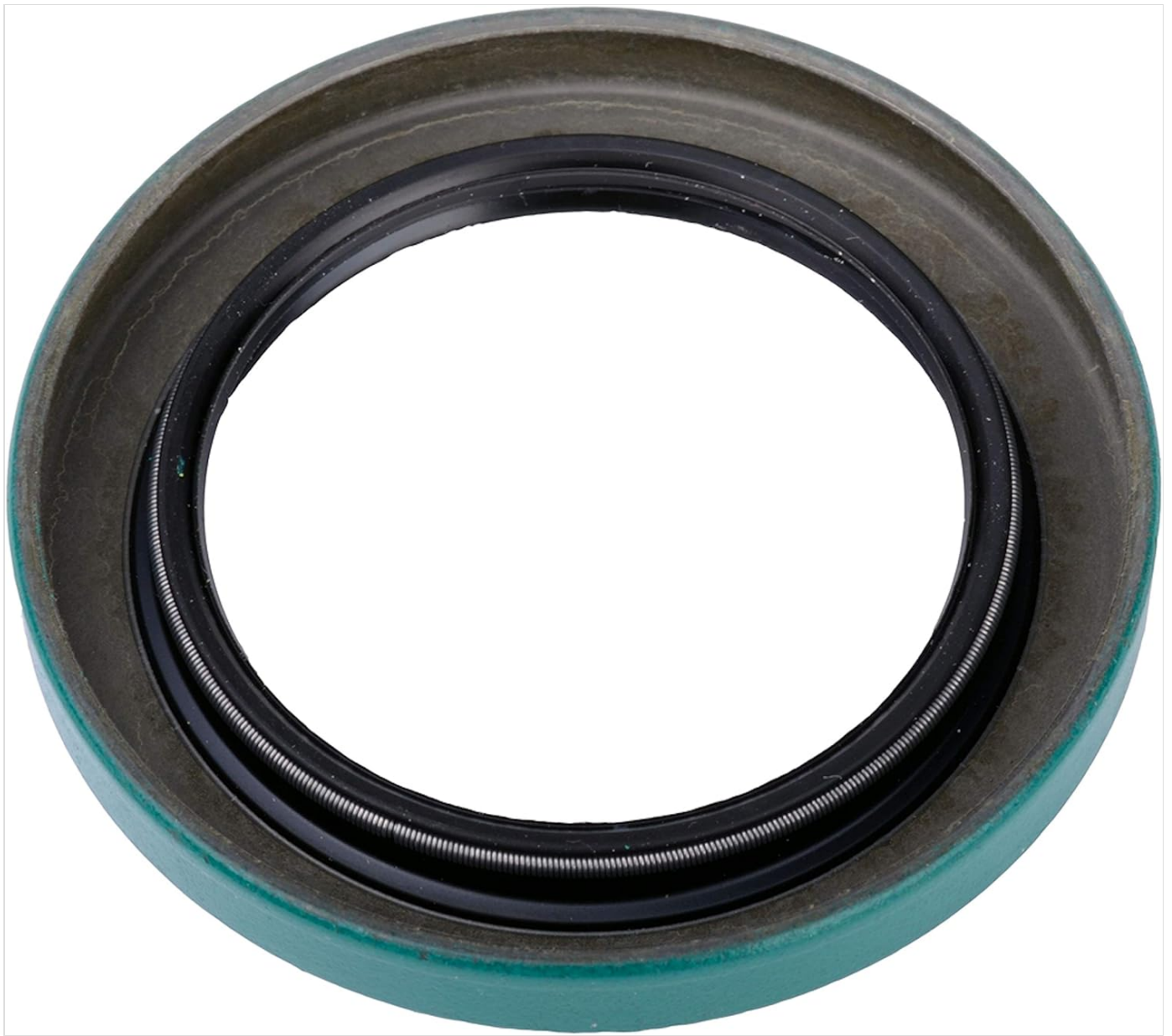
Figure 3.1: Front view of the SKF 17387 Power Steering Pitman Arm Shaft Seal. This image shows the primary sealing lip and the internal spring mechanism designed for consistent pressure against the shaft.
