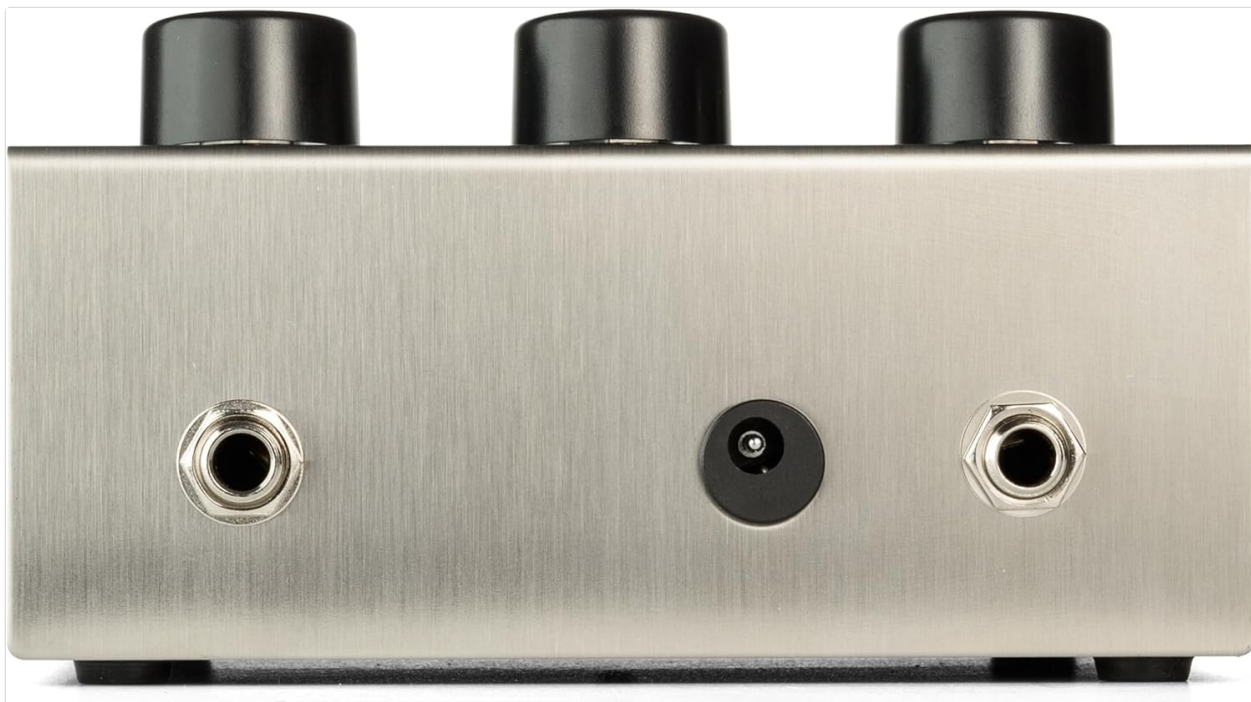
Figure 2: Top view of the Big Muff Pi, highlighting the input and output jacks for connection to your guitar and amplifier, and the power input.
