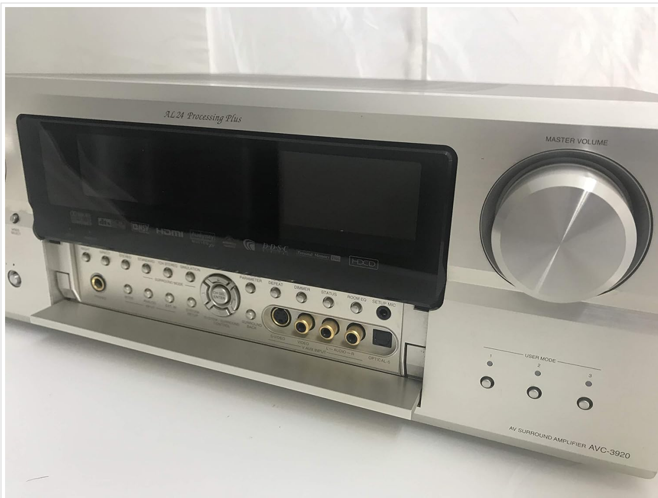
Figure 5.3: Right front panel controls, featuring the MASTER VOLUME knob and USER MODE buttons.
