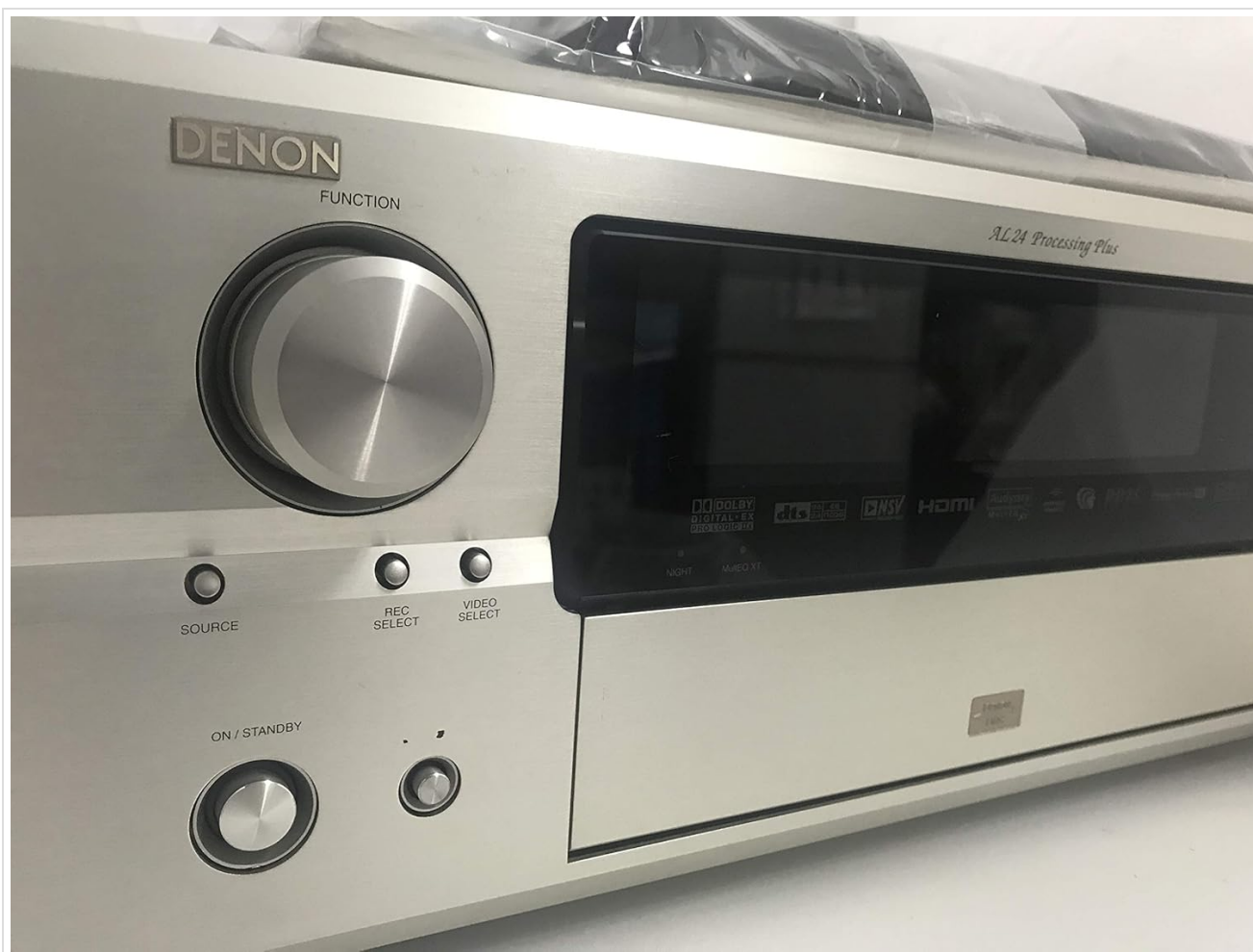
Figure 5.2: Left front panel controls, including the FUNCTION knob, SOURCE, REC SELECT, VIDEO SELECT buttons, and the ON/STANDBY button.
