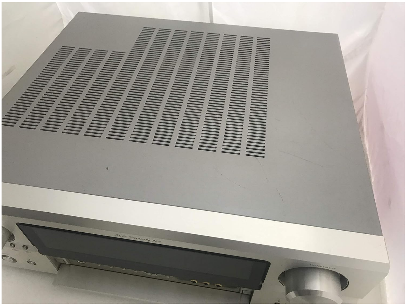
Figure 4.1: Top view of the AVC-3920SP, highlighting the ventilation grilles. Ensure these grilles are not obstructed to prevent overheating.
