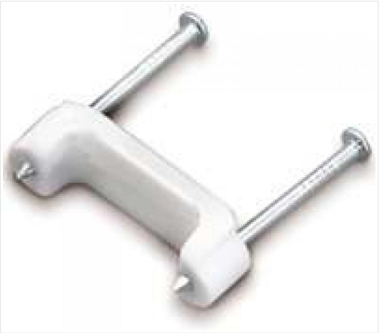
Figure 1: A single Gardner Bender PS-75 insulated staple, showing the white polyethylene saddle and two zinc-plated nails. This staple is designed to secure electrical cables to wooden surfaces.
