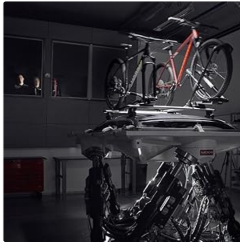
Figure 3.1: Example of bicycles secured on a Thule rack, illustrating how the no-sway cages contribute to overall stability during transport.
