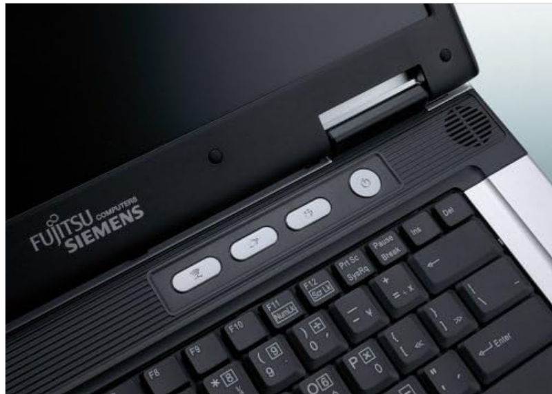
Image 3.2: A close-up view of the control buttons located above the keyboard on the Fujitsu AMILO A1650G, including the power button and quick-launch keys.
