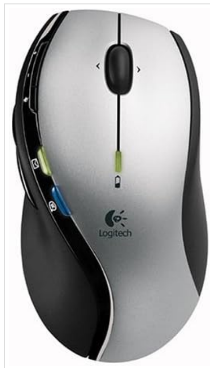
Figure 3: Top view of the MX 610 mouse, highlighting the scroll wheel and primary left/right click buttons.
