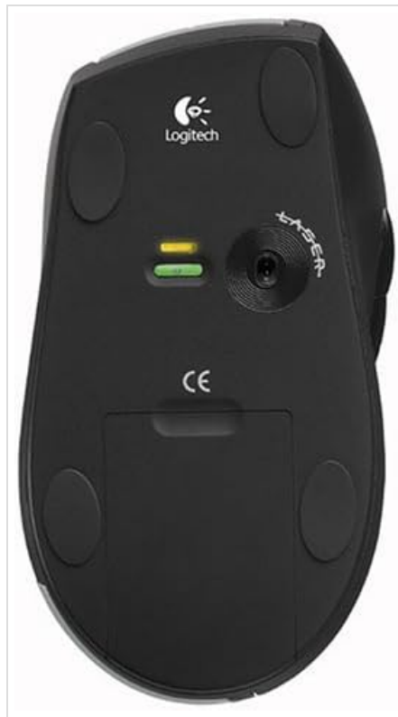
Figure 1: Underside of the MX 610 mouse with the battery compartment. The laser sensor is also visible.
