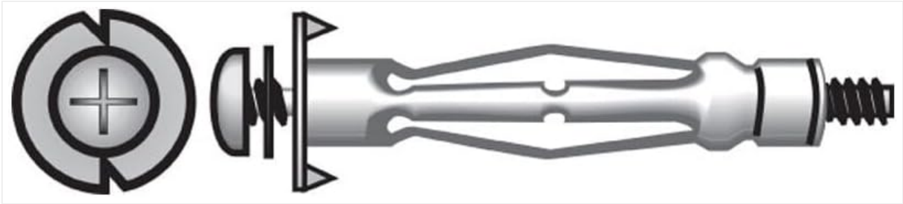
Image 5.1: Exploded diagram showing the anchor's components, including the screw, washer, and expanding body.
