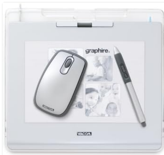
Figure 1: The Wacom Graphire4 6x8 USB Tablet, featuring its main components: the tablet surface, a cordless mouse, and a pressure-sensitive pen. The tablet surface includes a clear overlay for personalization and the 'graphire' logo.
