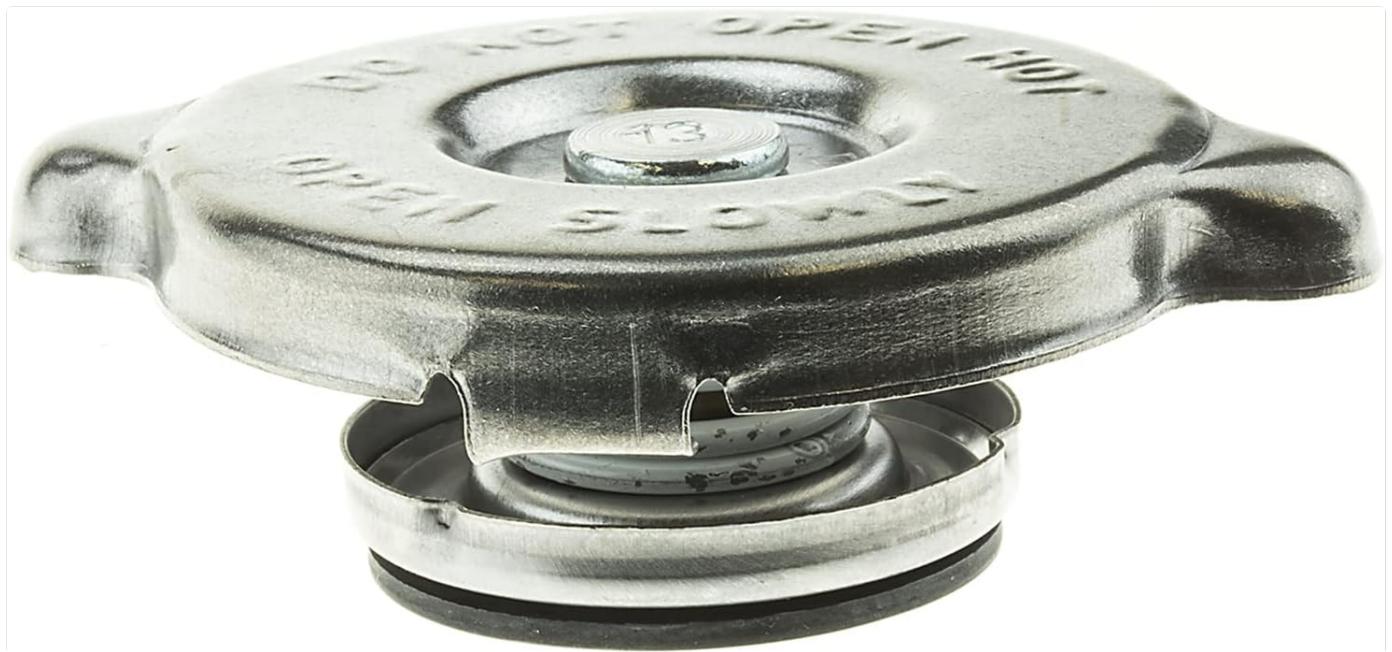
Image: Side view of the Stant Radiator Cap 10229, illustrating the internal spring mechanism and the lower rubber seal. This view is helpful for understanding how the cap creates a pressure seal within the radiator neck.
