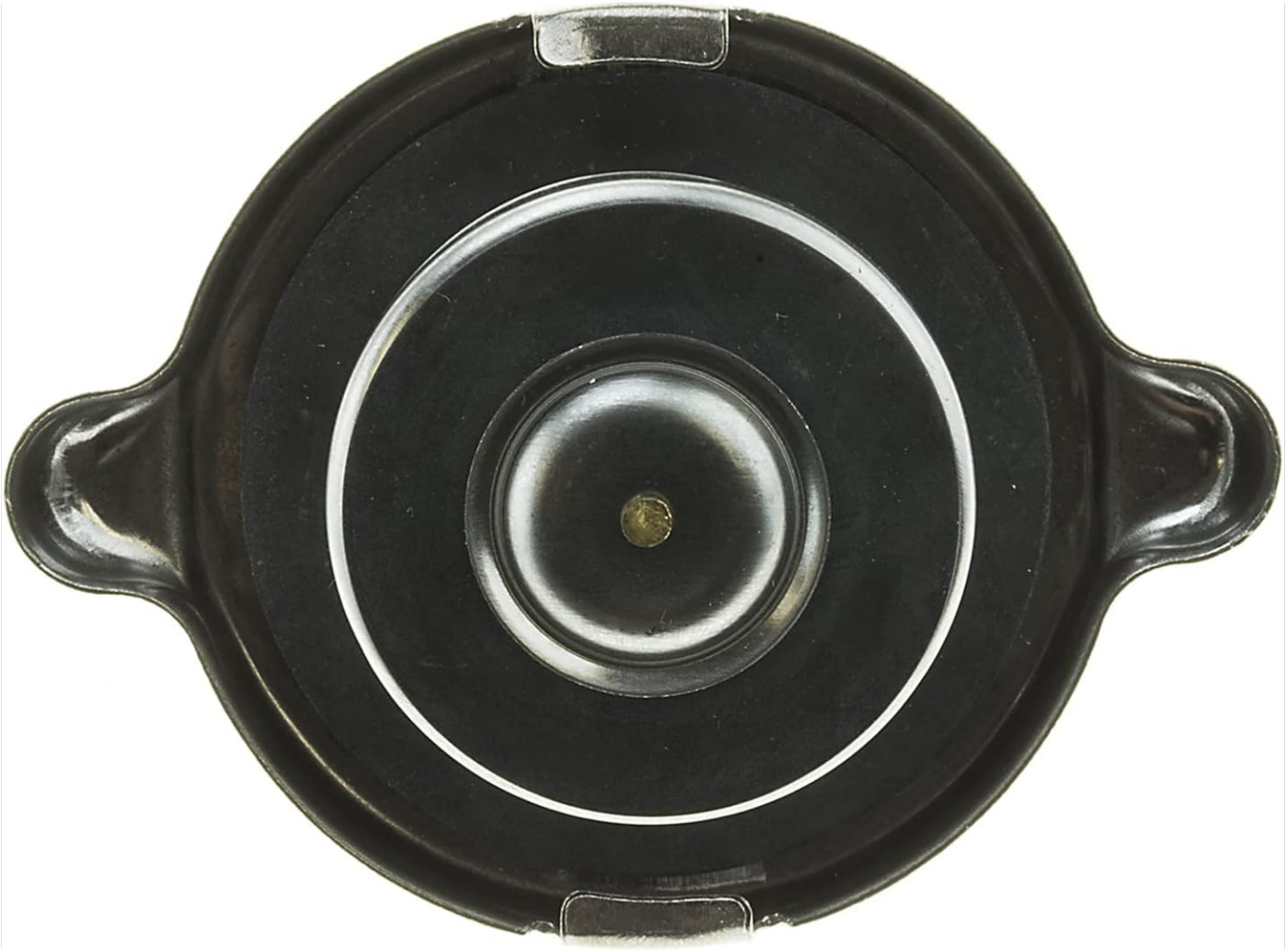
Image: Bottom view of the Stant Radiator Cap 10229, clearly showing the main rubber seal that creates the pressure seal against the radiator neck, and the smaller vacuum valve in the center. This view is critical for inspecting the integrity of the sealing components.
