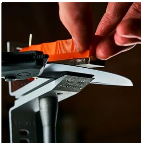
Image: Demonstrating the sharpening process with a Lansky hone and knife clamp.
