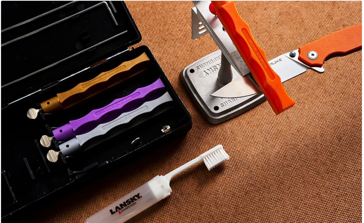
Image: All components of the Lansky 4-Stone Deluxe Diamond Sharpening System in its case.
