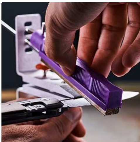
Image: Close-up of the Lansky knife clamp, highlighting the angle selection holes.
