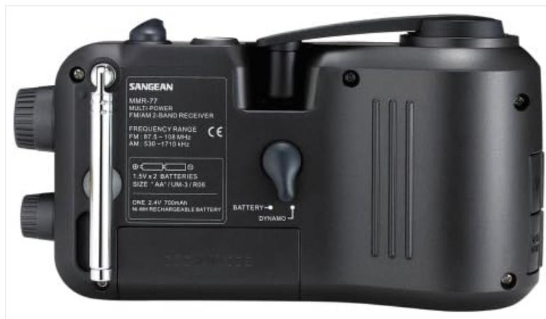
Rear view of the Sangean MMR-77, illustrating the battery compartment and the dynamo crank mechanism.
