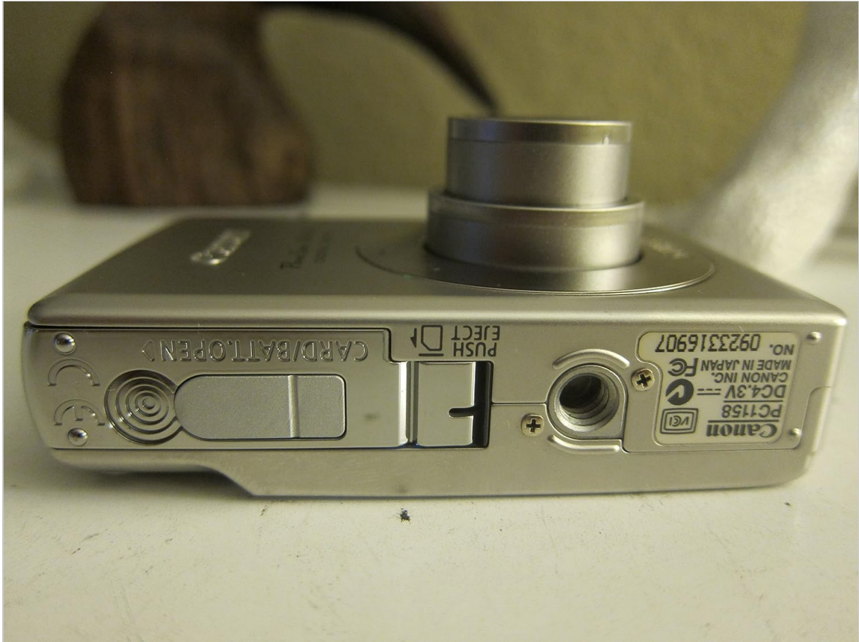
Figure 3.1: Bottom view of the camera, illustrating the battery and SD card compartment.
