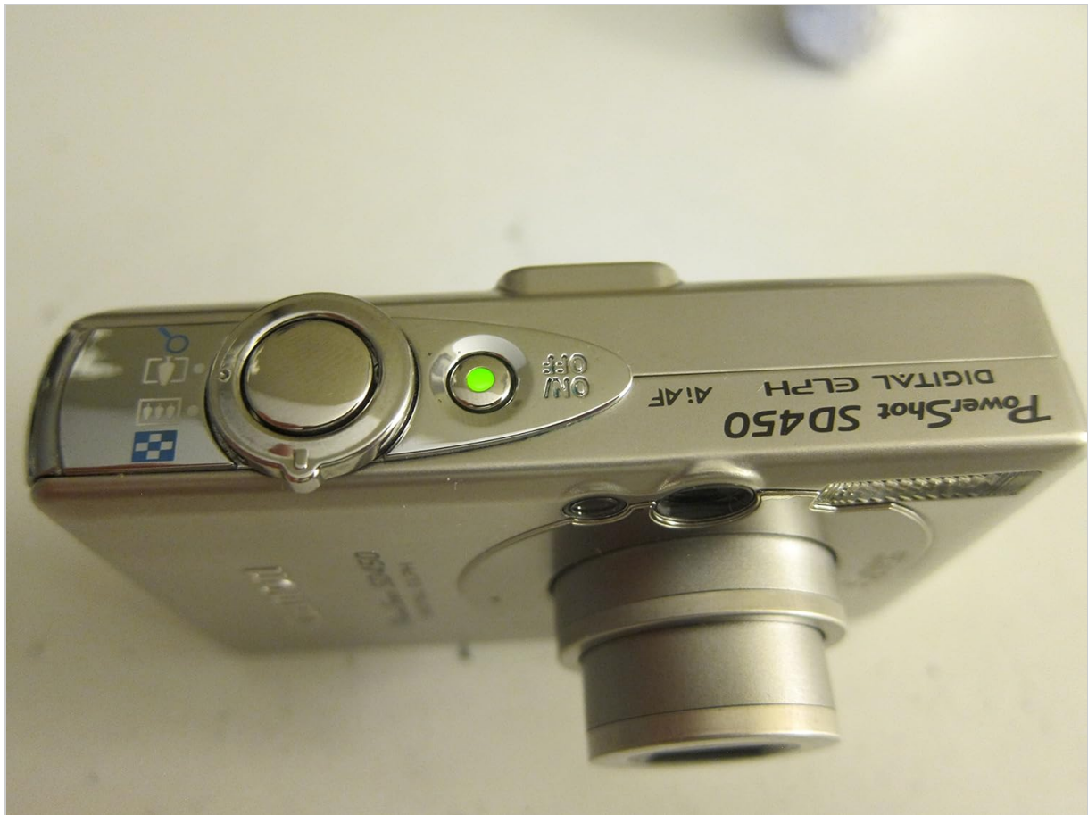
Figure 3.2: Top view of the camera, highlighting the power button and shutter release.
