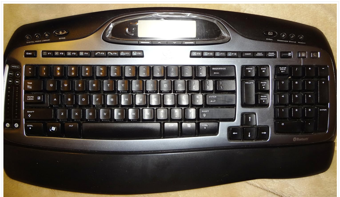
Image: Close-up view of the Logitech MX 5000 keyboard, showing the LCD display, touch-sensitive media controls, and key layout.
