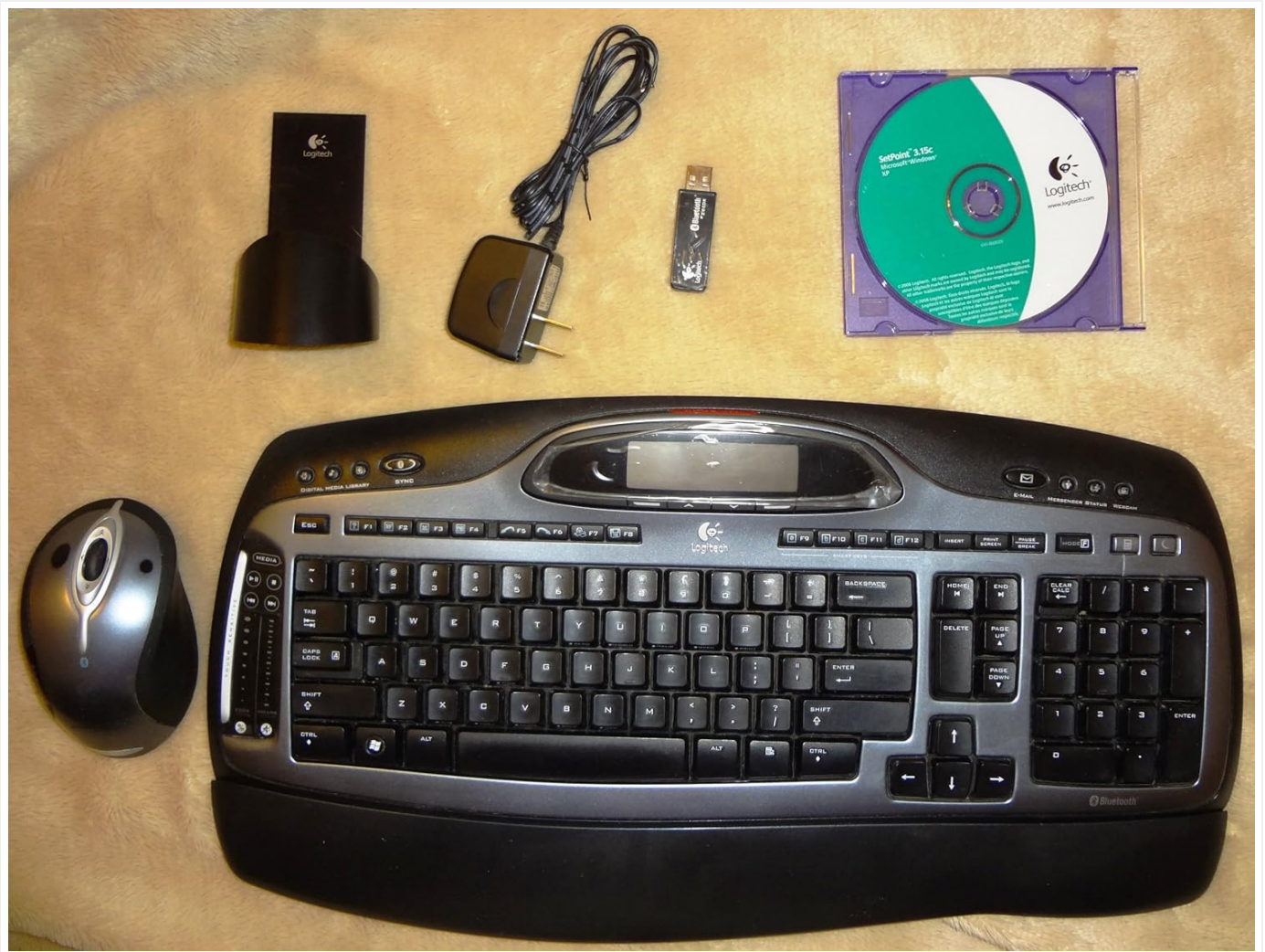
Image: All components of the Logitech Cordless Desktop MX 5000 Laser, including the keyboard, mouse, USB Bluetooth mini-receiver, rapid-charging base station, AC adapter, and software CD.
