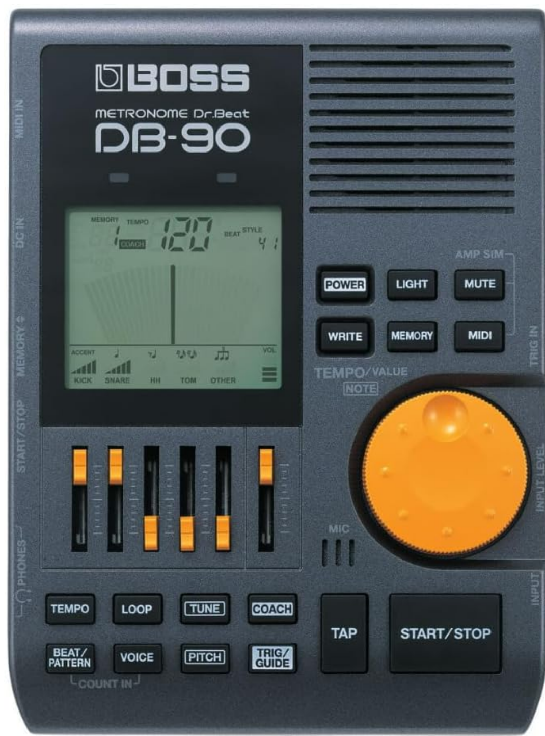
Figure 1: Front panel of the BOSS DB-90 Dr. Beat Metronome, showing the LCD screen, control buttons, sliders, and rotary dial.
