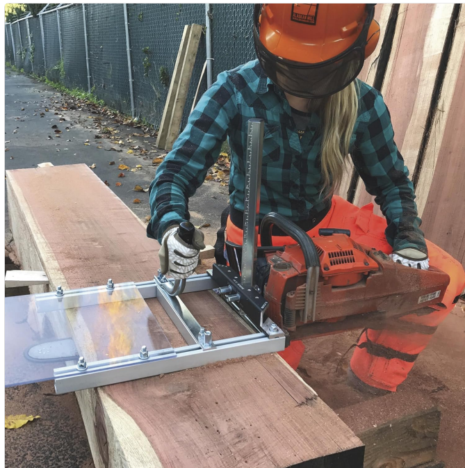
Figure 4: A person operating the Granberg G777 mill on a log, utilizing a guide rail for the initial cut.
