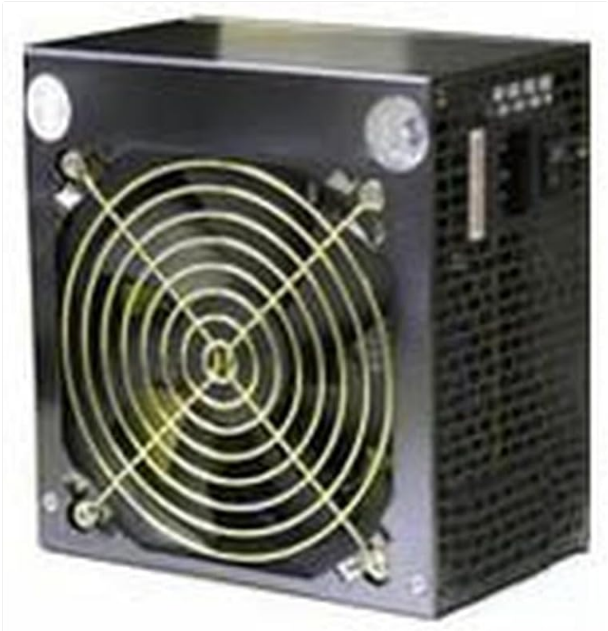
Figure 4.1: Front view of the power supply with its 120mm fan.
