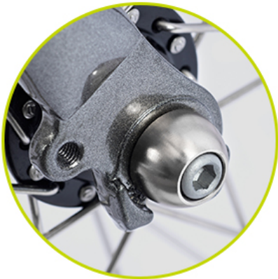
Figure 3.2: The Axlerodz skewer head, demonstrating compatibility with standard 9mm dropouts.
