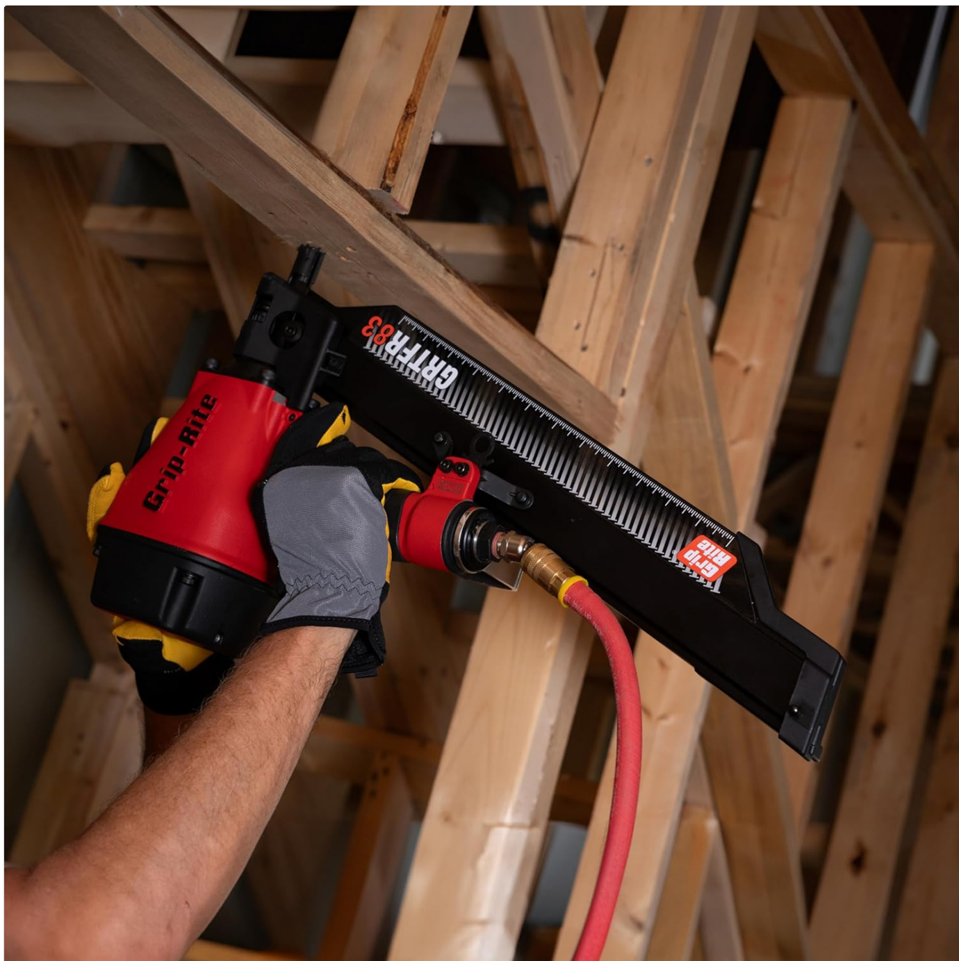
Image: A construction worker operating a Grip-Rite framing nailer to fasten lumber, illustrating the typical application of these nails in a building project.
