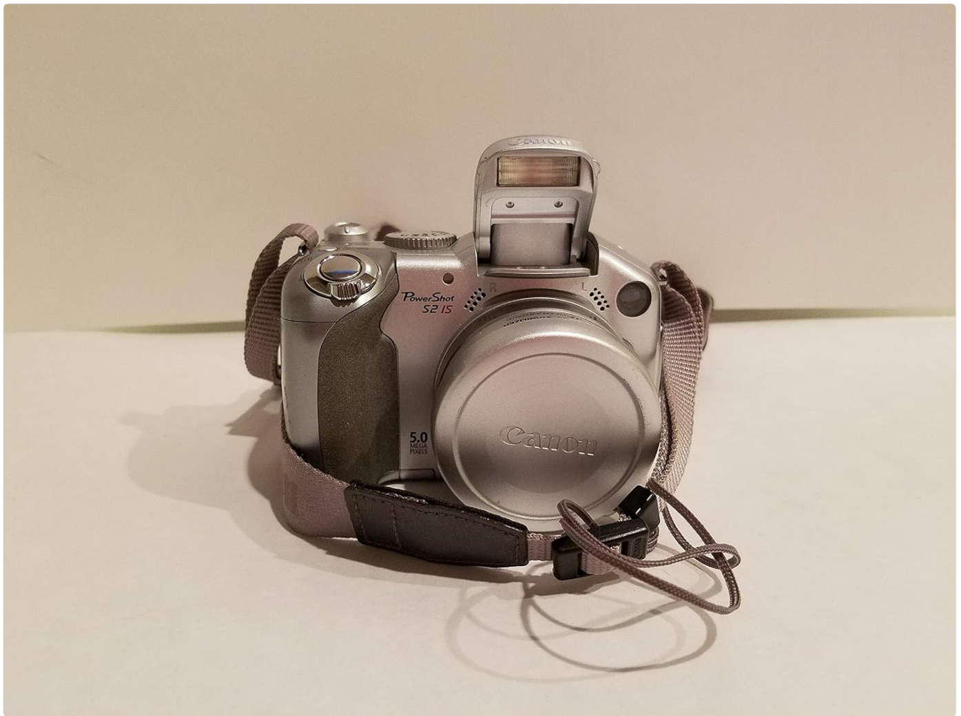
Figure 4.2.1: Front view of the Canon PowerShot S2 IS camera with the built-in flash popped up, ready for use in low-light conditions.
