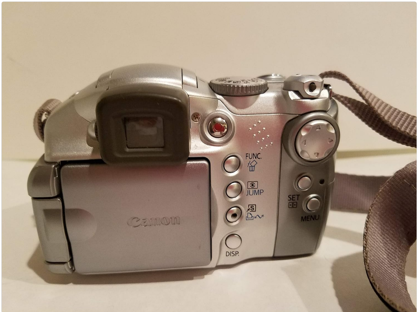
Figure 4.1.1: Rear view of the Canon PowerShot S2 IS camera, showing the closed vari-angle LCD, the electronic viewfinder, and control buttons including FUNC, JUMP, SET, MENU, and DISP.
