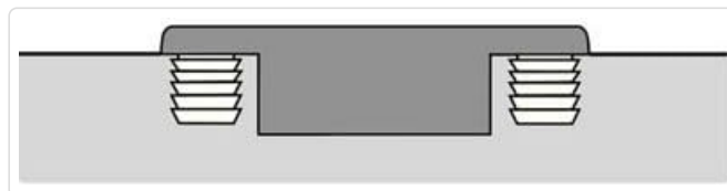
Image: Cross-section diagram showing the hinge cup installed within the cabinet door, illustrating the concealed nature of the hinge.
