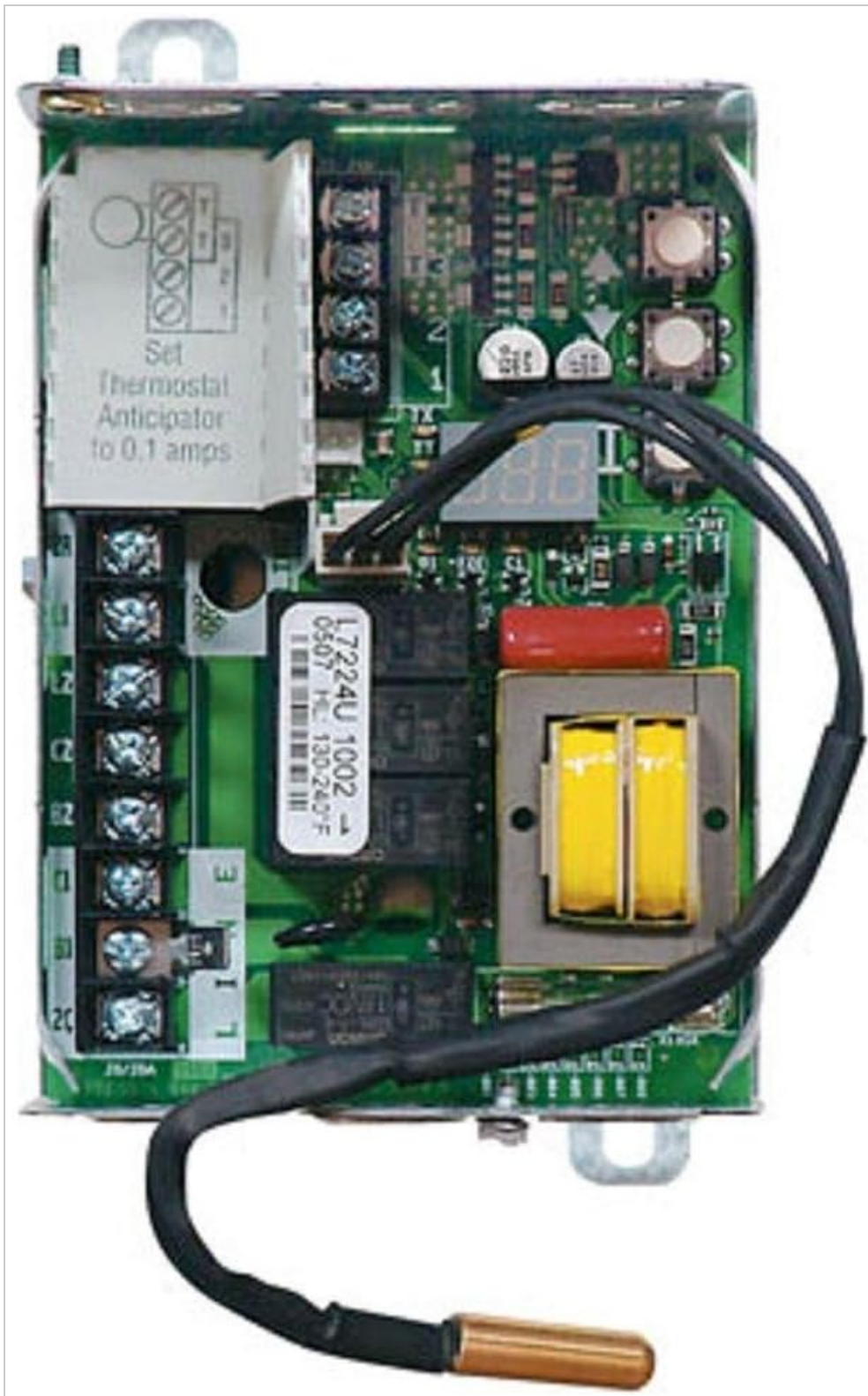
Figure 2: Internal view of the Honeywell L7224U-1002 Aquastat circuit board. This image displays the electronic components, wiring terminals, relays, and the LED display, highlighting the device's internal complexity and connection points for various system components.
