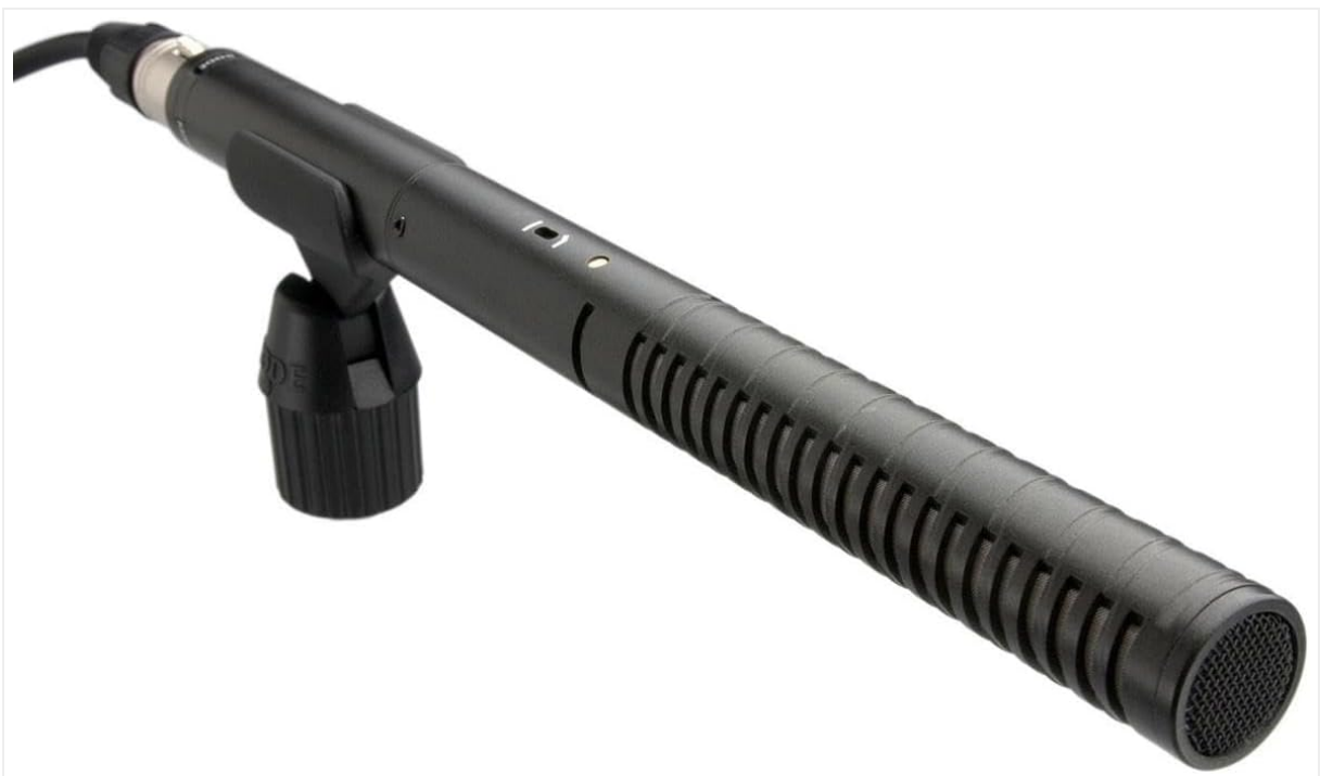
Figure 2: A close-up view of the Rode NTG-2 microphone body, clearly showing the switch for the 80Hz high-pass filter. This switch allows users to reduce low-frequency noise.
