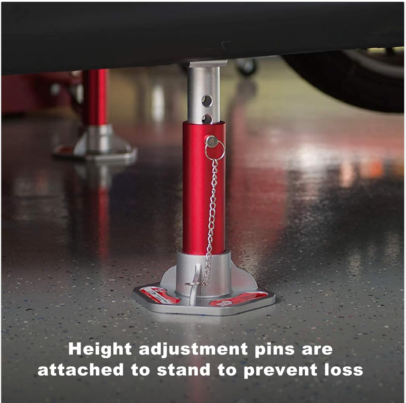
Image: A close-up view of the height adjustment mechanism of the jack stand, showing the locking support pin securely inserted through the inner and outer columns.
