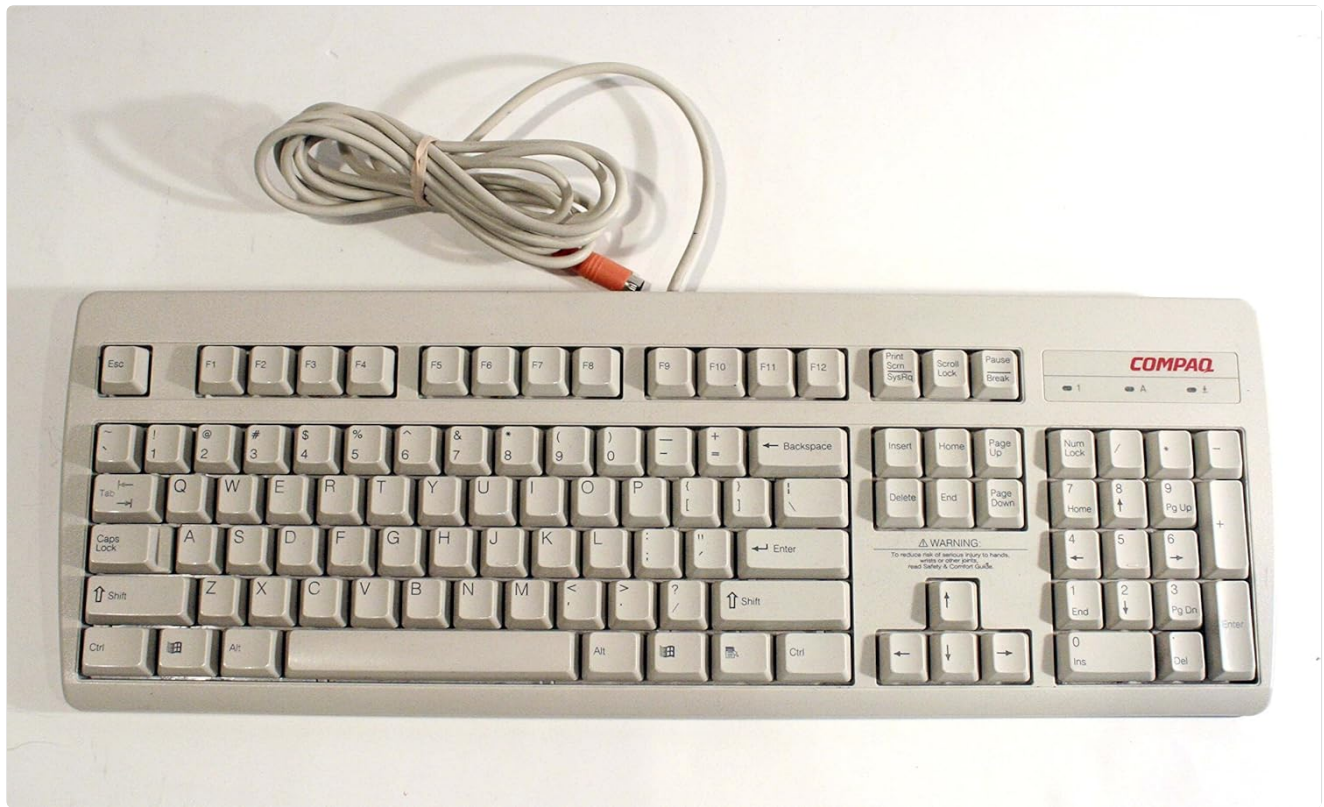
Figure 2.2.1: Top-down view of the Compaq KB-0133 PS/2 Keyboard, illustrating the key layout and PS/2 cable.
