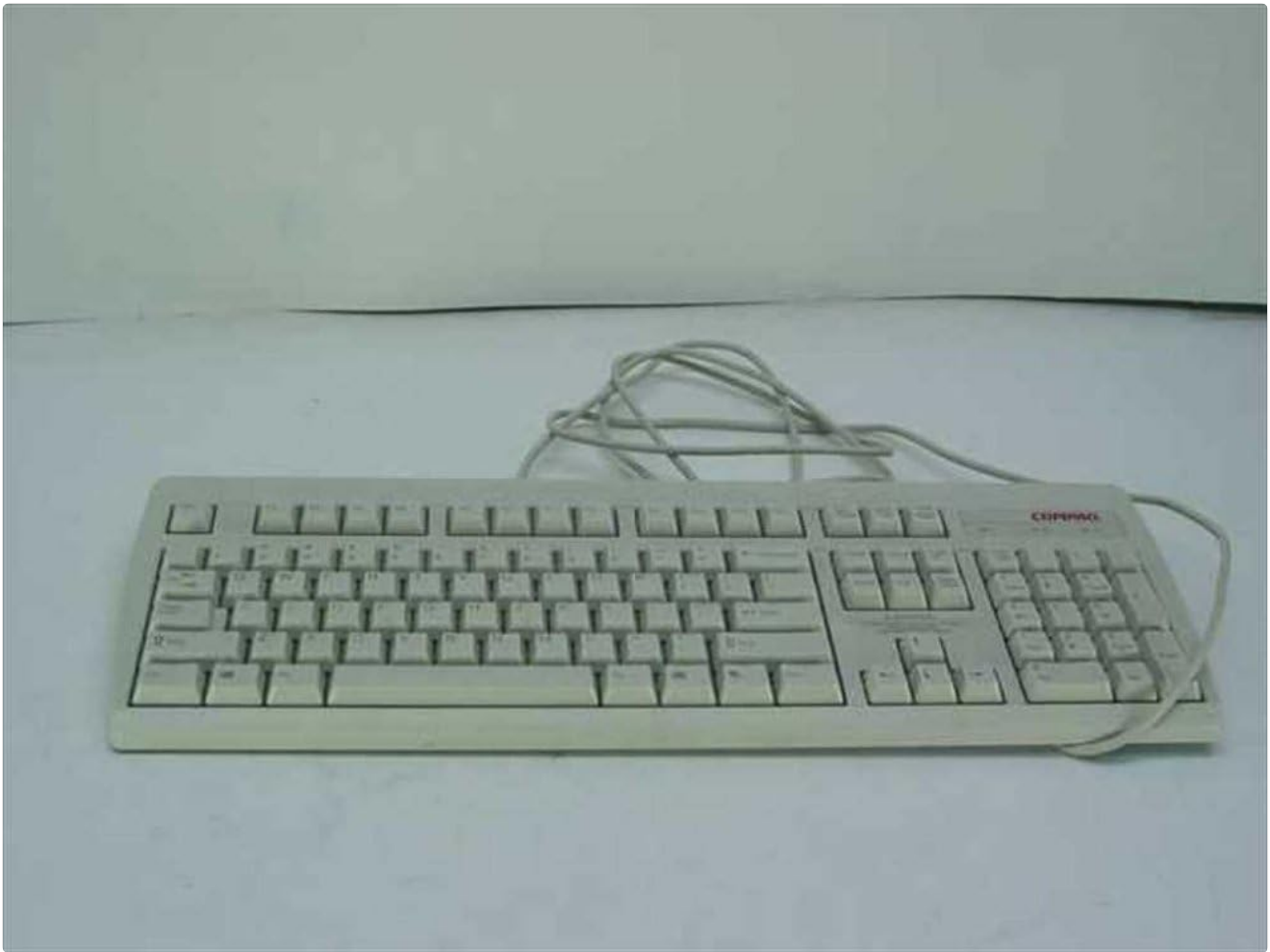
Figure 3.2.1: Angled view of the Compaq KB-0133 PS/2 Keyboard, showing the hot keys.
