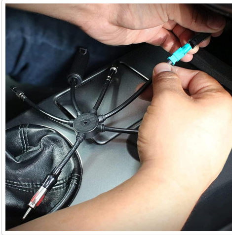
Image: A hand connecting the standard male DIN connector of the UAA3 adapter to the antenna input on an aftermarket car stereo.
