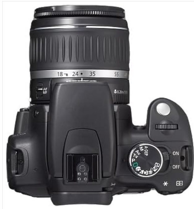
Figure 2: Top view of the camera, showing the lens mount and mode dial.
