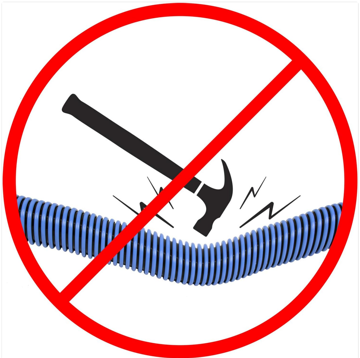
Figure 5.1: Avoid crushing or bending the hose sharply to maintain its integrity and prevent damage.
