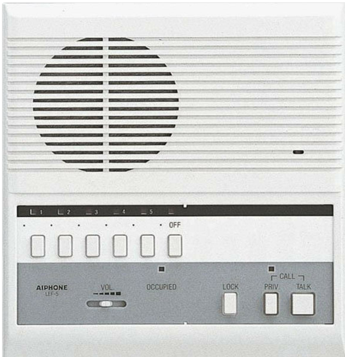
Image 1: Front view of the Aiphone LEF-5 Master Intercom. The unit features a large speaker grille at the top. Below the speaker, there are five numbered call buttons (L1, L2, 3, 4, 5) with an 'OFF' indicator. A volume slider labeled 'VOL' is located on the left side of the control panel. An 'OCCUPIED' indicator is centrally located. On the right, there are three push buttons: 'LOCK' for door release, 'PRIV' for privacy, and 'TALK' for communication, with a 'CALL' indicator above the 'PRIV' button.
