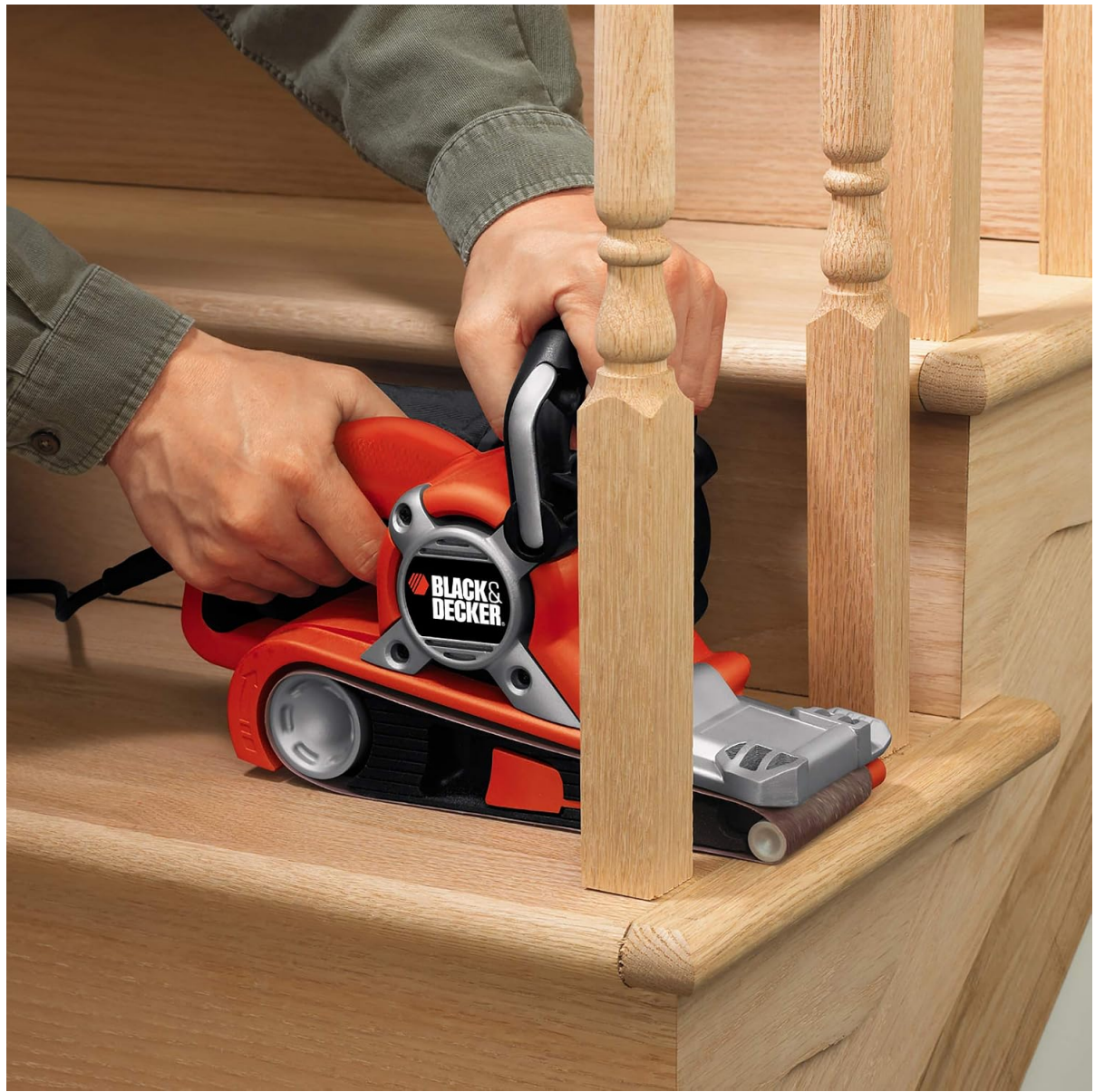
Figure 6: The sander being used on stair balusters, demonstrating its versatility for various woodworking tasks.
