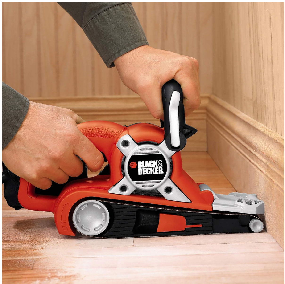
Figure 4: Demonstrating close-edge sanding, utilizing the front roller for precision near baseboards.
