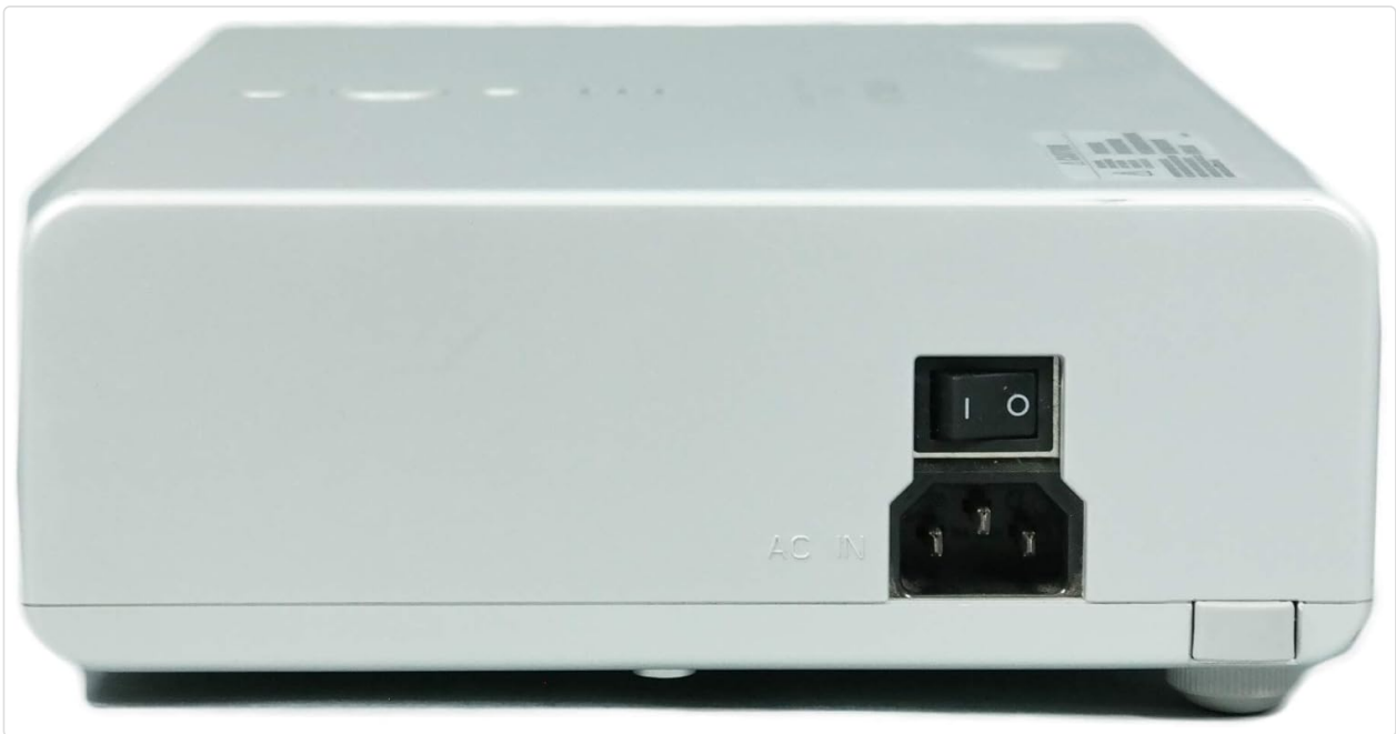
Image 3: Side view of the Hitachi CP-RS55 projector. This image focuses on the side panel, clearly showing the 'AC IN' power receptacle and the main power toggle switch located above it.
