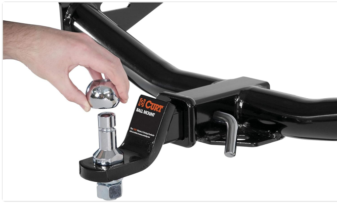
Image 1: Position the Switch Ball head directly above the Switch Ball shank on your ball mount. Ensure the shank is clean and free of debris.
