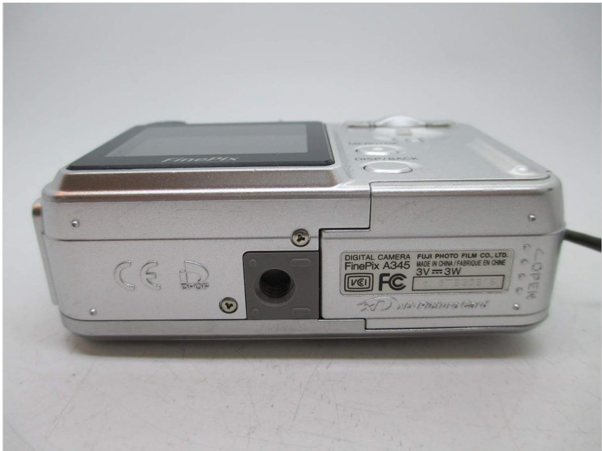
Image: Bottom view of the Fujifilm Finepix A345 camera, illustrating the battery and xD-Picture Card compartment. The 'OPEN' indicator is visible near the latch.
