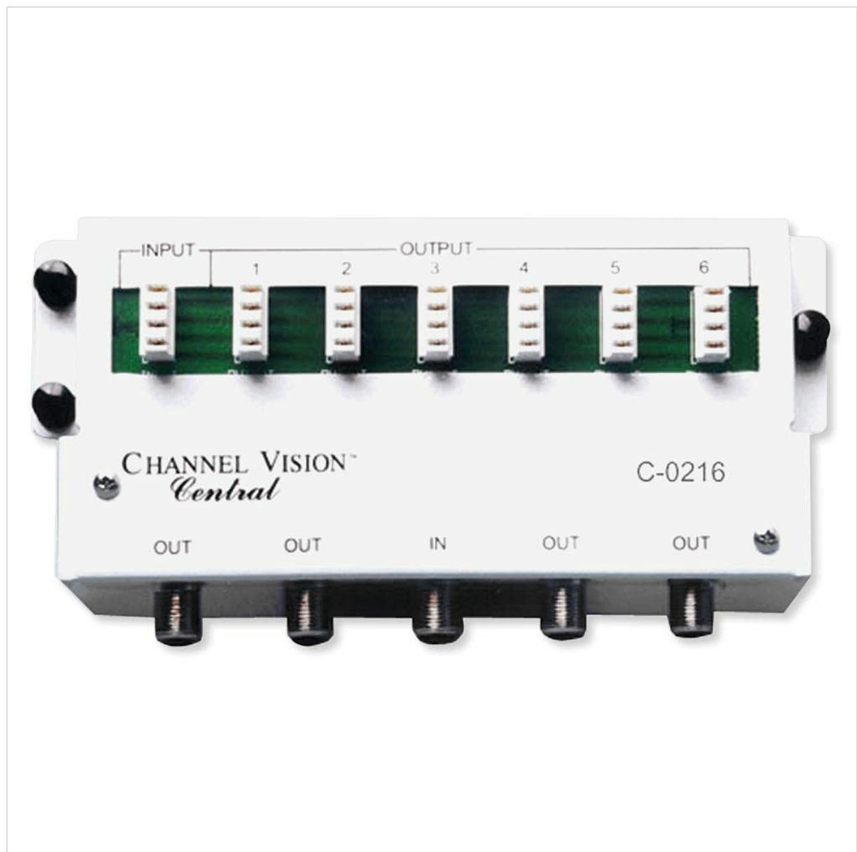
**Figure 1:** Front view of the Channel Vision C-0216 module. The top section shows the 110 punch down block with "INPUT" and "OUTPUT" labels for telephone lines 1 through 6. The bottom section displays coaxial F-connectors labeled "OUT", "OUT", "IN", "OUT", "OUT" for RF signal distribution. The model number C-0216 is visible on the right side.
