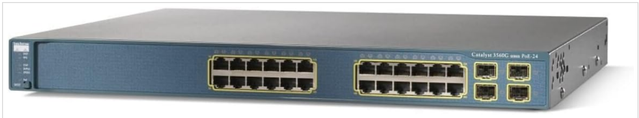
Figure 1: Front panel of the Cisco Catalyst 3560G-24PS-S Switch. This image displays the front panel of the Cisco Catalyst 3560G-24PS-S switch, featuring 24 Gigabit Ethernet ports with Power over Ethernet (PoE) capability and four SFP (mini-GBIC) uplink slots on the right side. The left side shows status indicator LEDs and a console port.
